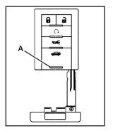
To remove the key, press the button (A) near the bottom of the keyless access transmitter, and pull the key out. Never pull the key without pressing the button.
